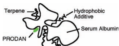
Figure 1. Schematic illustration of the proposed sensing ensemble, composed of the indicator PRODAN, terpene, and a hydrophobic additive, all of which are added to the serum albumin protein. 4d
